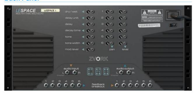
The back panel exposes the input / output CV (Control Voltage) and audio output sockets.
